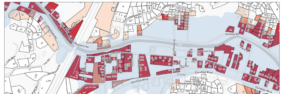
Figure 17. Community asset-level map with higher levels of combined vulnerability and risk for parcels in darker red. Source: Fernleaf.
